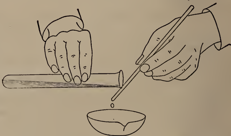
Fig. 7. Pouring a liquid down a glass rod.
